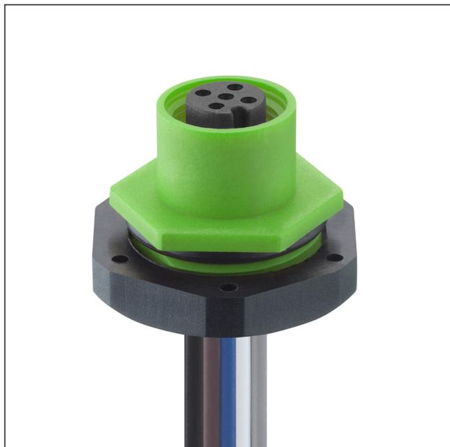
M12 panel mount connector, female, A-coded, IP67, for front mounting, thread M20, with nut and stranded wires, with plastic housing, green
