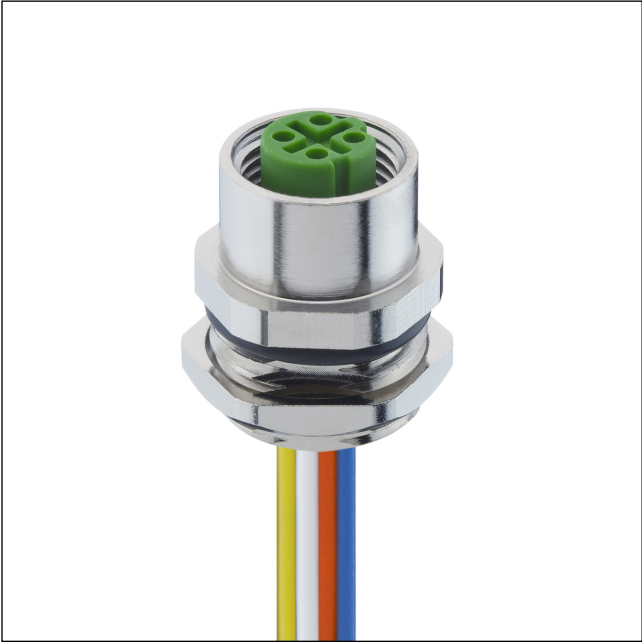
M12 panel mount connector, female, D-coded, IP67, for front mounting, thread M16, with nut and stranded wires
